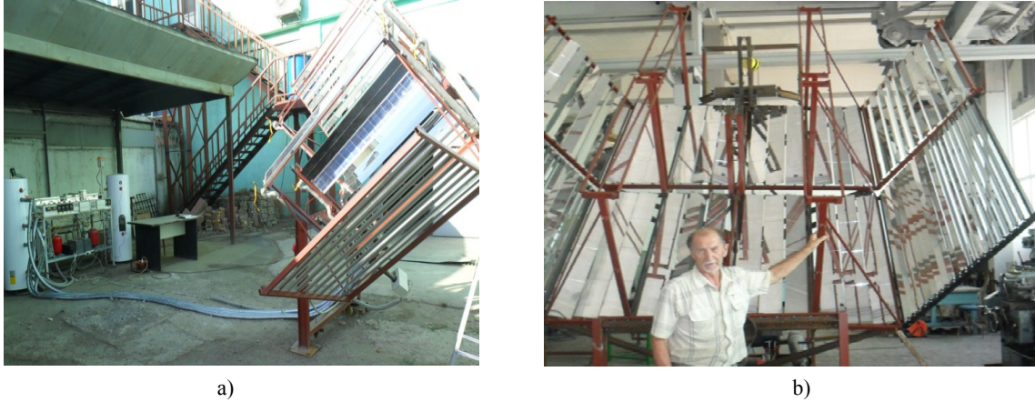
FIGURE 1. Laboratory model of CPVT system; a) experimental stand for testing b) assembly of the concentrator mirrors.
