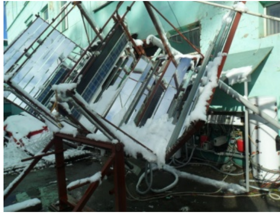
FIGURE 5. Snow melting on the surfaces of carrier platform mirrors.
